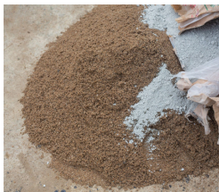
Mortar Materials Portland, Sand, Water
