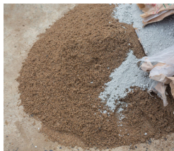
Mortar Materials Portland, Sand, Water
