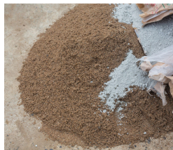
Mortar Materials Portland, Sand, Water
